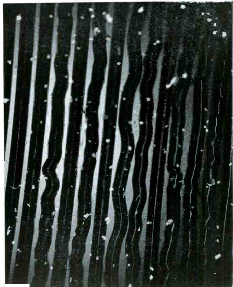
Lint particles removed from wiping cloth by sharp groove edges of freshly cut disc.
