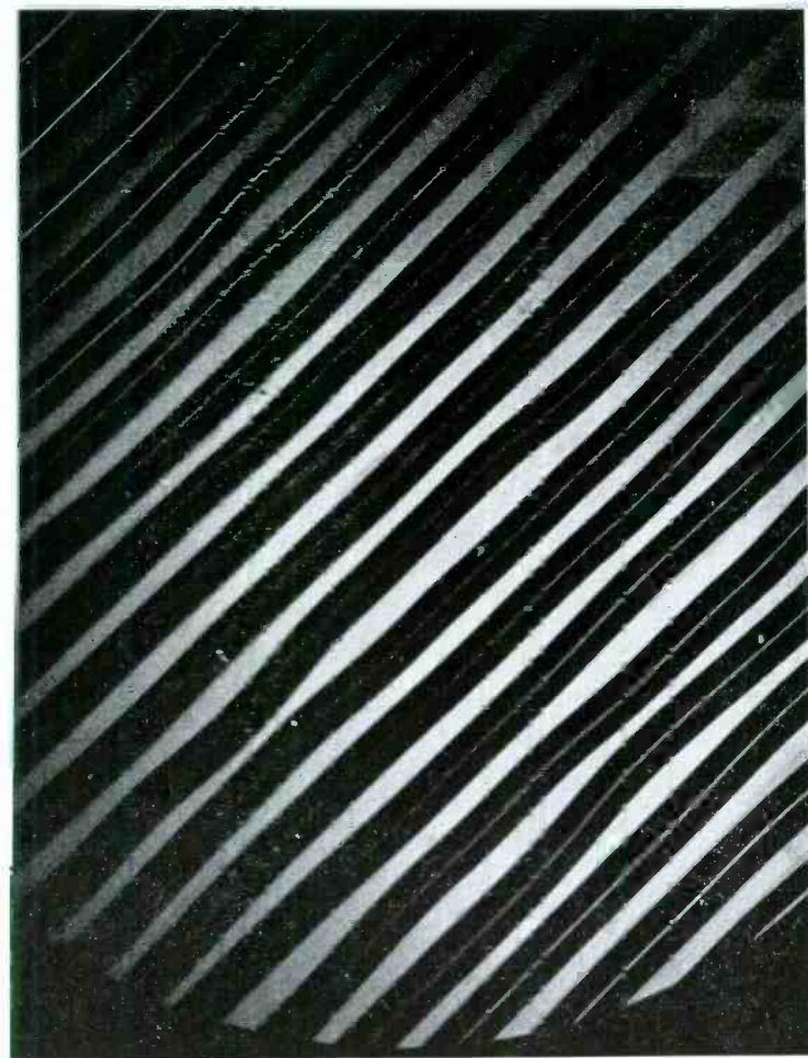
Normal cut (60% groove width, 40% "land" between grooves) with normal modulation. Average program material.
